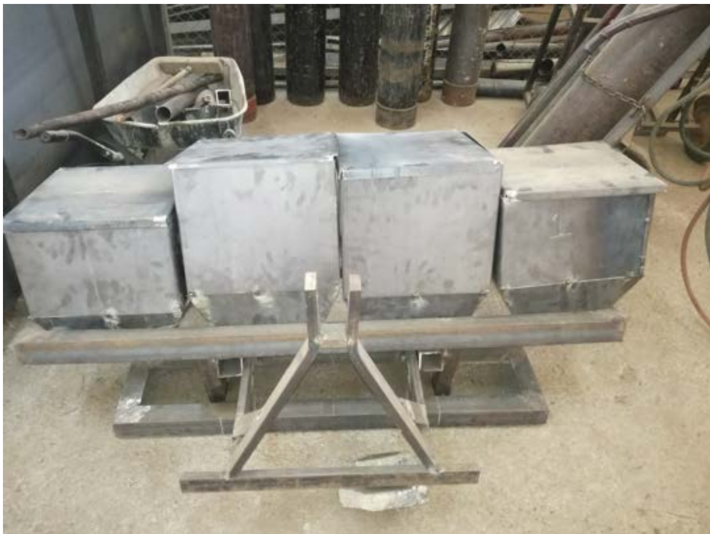
Figure 14. Prototype of safflower planter with chamber for fertilizer application.
